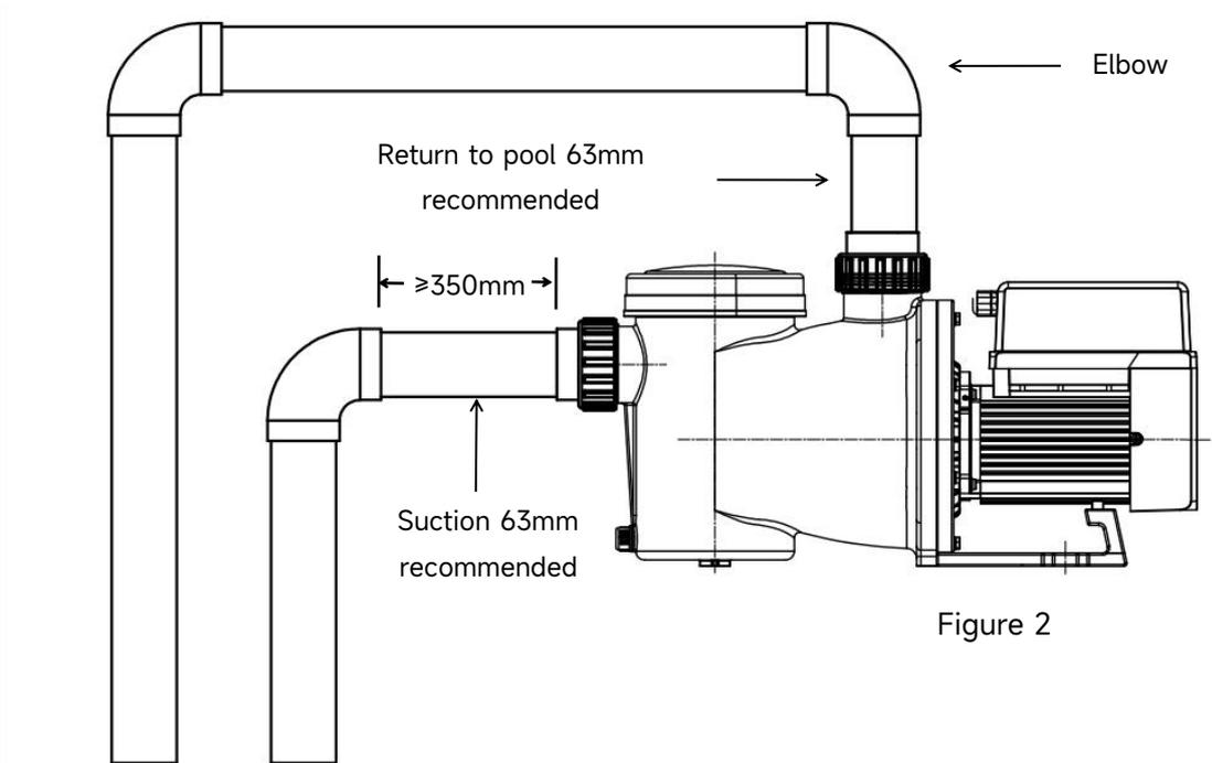
\* The pump inlet/outlet union size: optional with 48.5/50/60.3/63mm
